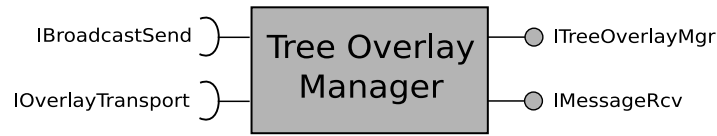
Figure 3: The TOM Component with its Interfaces and Receptacles.
